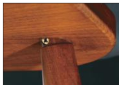
Legs and Stretchers Reinforced with Screws
